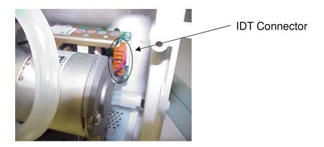
that the pump will run to ensure proper placement of the battery wires. In addition, make sure IDT connector is placed in correct position.
